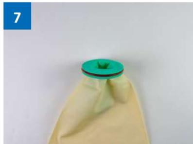
7 Take the silicone rubber O-ring and fix into groove of connector over the glove
