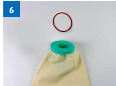
6 Continue as in photo #5, ensuring to completely cover the sleeve cuff connector with the cuff of the glove
