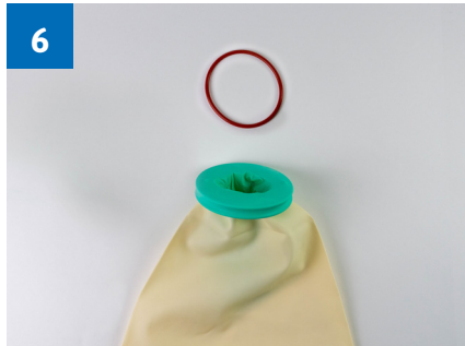
Continue as in photo #5, ensuring to completely cover the sleeve cuff connector with the cuff of the glove
