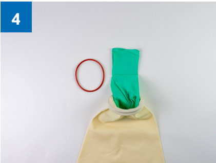
Take the glove and feed it through the cuff connector, fingers first
