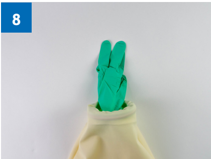
Turn the assembled sleeve and glove the correct way round
