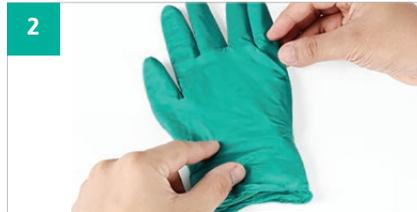
2 Remove one glove from the package and inspect it to be sure no pinholes or tears are present.
