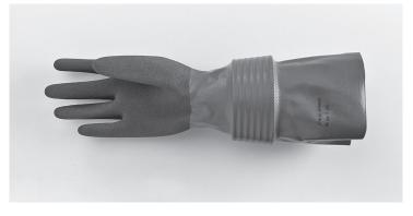
Step 2 - Ensure the glove fully covers the grey cone.
