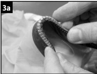
b) A broken zipper has a V-shaped bend.
