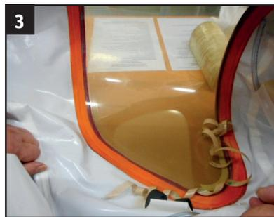
4) Finally, press the taped edge carefully against the visor. Use your hand or a roller.
