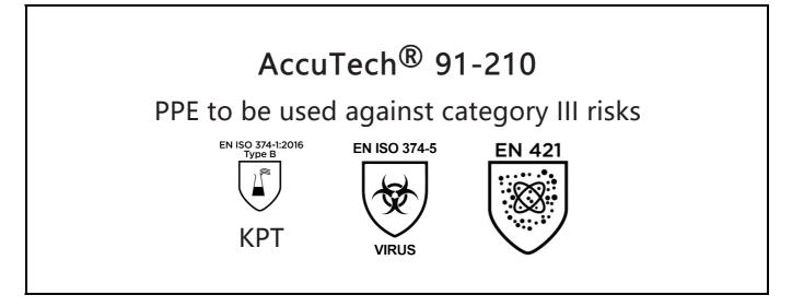
is in conformity with the provisions of Regulation (EU) 2016/425 and with the standards EN 420:2003 + A1:2009, EN ISO 374-1:2016 Type B, EN ISO 374-5:2016, EN 421:2010 and is identical to the PPE which is subject to the EU-Type examination (Module B, Annex V of the Regulation), under certificate number 032/2020/1042, issued by the Notified Body:
