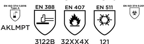
is in conformity with the provisions of Regulation (EU) 2016/425 and with the standards EN ISO 374-1:2016, EN 388:2016, EN 407:2004, EN 420:2003 + A1:2009, EN 511:2006, EN ISO 374-5:2016 and is identical to the PPE which is subject to the EU-Type examination (Module B, Annex V of the Regulation), under certificate number 032/2018/2167, issued by the Notified Body:
