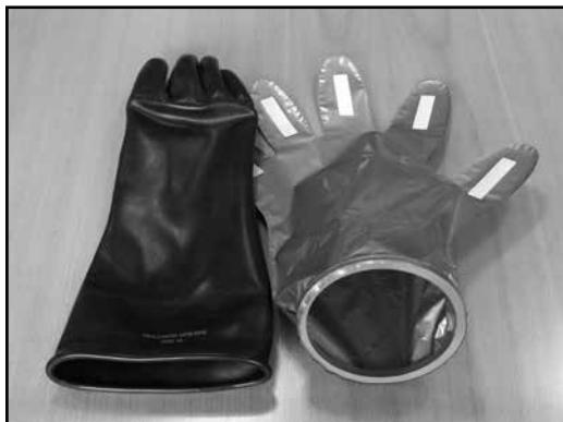
2. Remove the white protective film on each finger of the inner glove. This will uncover a sticky area that will hold the inner glove in place and keep it inside the outer glove when the hand is retracted.
