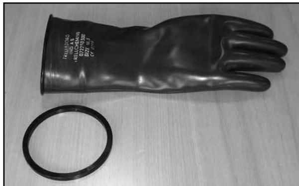
1. Push the black inner ring into the glove. Position it approximately 5 cm (2 inches) into the glove.
