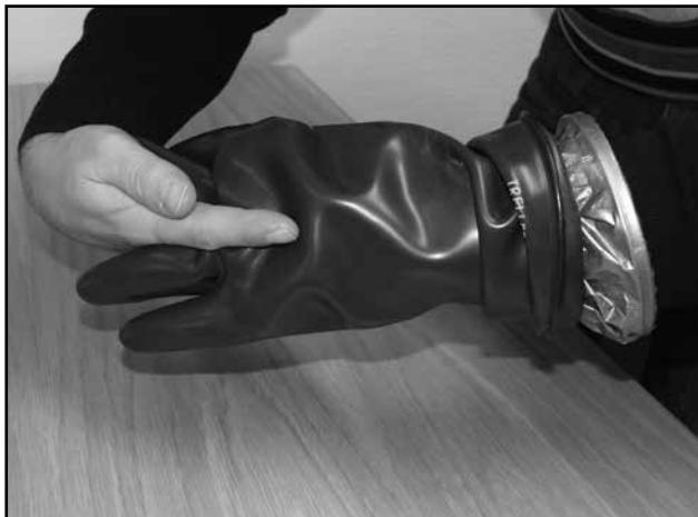
3. Push the inner glove into the outer rubber glove. Make sure all fingers of the inner glove come into position all the way inside the fingers of the outer glove.
