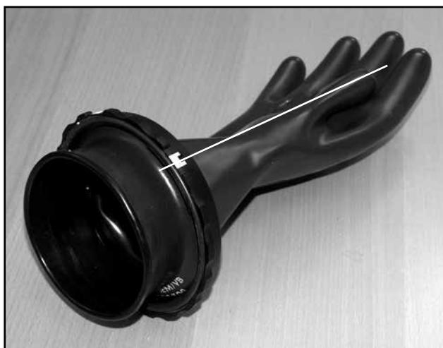
8. The gloves can be detached by going through the applicable steps above “backwards”. The inner glove will stick to the outer glove but this can be overcome by using a little force. You may try one finger at a time and/or turning the outer glove inside-out if you have problems detaching the inner glove.
