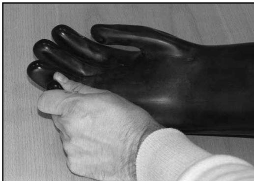
4. Press the fingers of the outer and inner gloves together so that they stick together.
